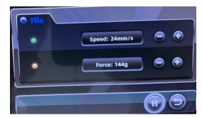
"File" icon is specially used to adjust cutting speed and force during working. Also used for give a demand of pause to machine.
