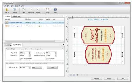
To control the position of each logo, you can use the "Job Position (x)" property. If for example, you want both labels to be aligned to the right, you would select both of them (using the shift key to multiple select), and then select "Right" as the positioning option, and enter the desired value that both of the logos right edge ends up as.
