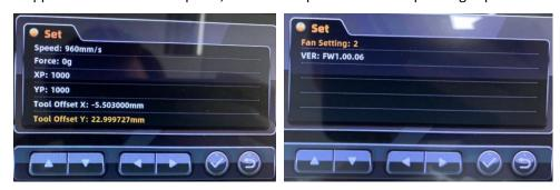
"Set" icon is to adjust configurations or functions such as speed, force, fan level etc. Usually enter this interface before process rolls.
