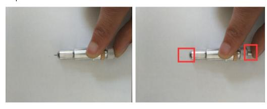
The tip of the blade depends on the length of the cutting material thickness
