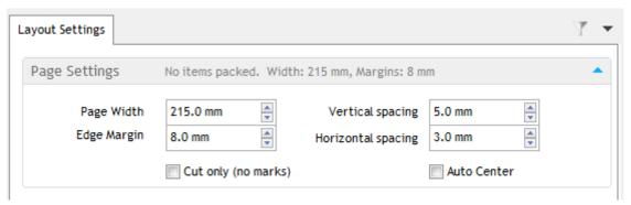
**Paper Width:** Total size of printed artwork. This should be slightly less than the maximum printing size of your printer.
