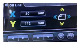
"Off Line" icon is used to remove cutting head/red light to expected position such as cut blank sticker or scan mark before cutting.
